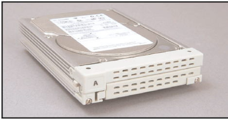
Removable RAID drives for security requirements.
